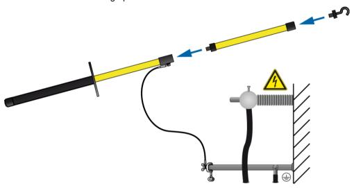
3. Use the black handle to hold the discharge and earth rod and make contact with the test object by touching it with the tip of the discharge and earth rod.
