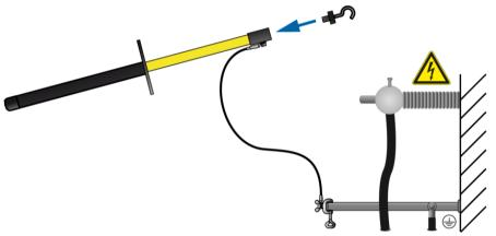
3. Contact the test object with the tip of the earth rod.
