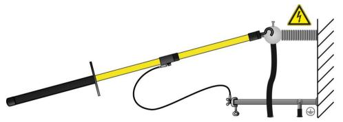
4. Observe the minimum discharge period in accordance with the capacitance of the test object.
