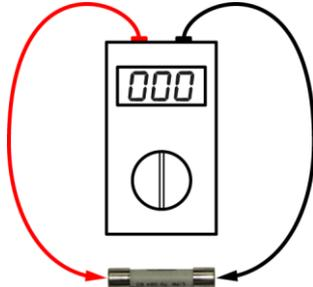
Check if the fuse is working. For this, perform a continuity check with a multimeter.
