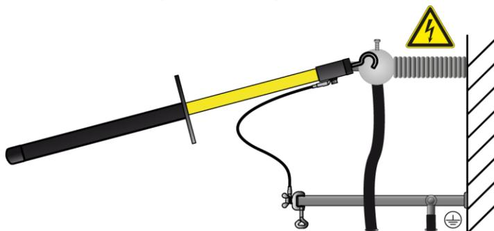
4. Immediately after earthing, connect the earthing and short-circuit equipment to the test object.
