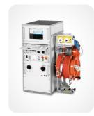
↑ 03 / Syscompact 4000 cable fault location system
