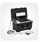
**07 /** Time domain reflectormeter IRG 4000 portable
