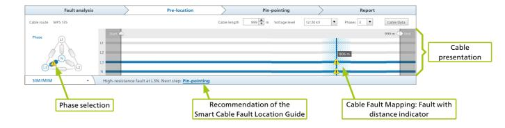
BAUR Software 4 – cable fault location
