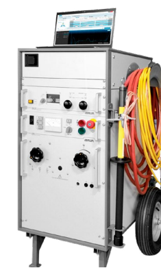
↑ Syscompact 400 portable is used for cable fault location and is very well suited for mobile use, without the need for a permanent vehicle installation.
