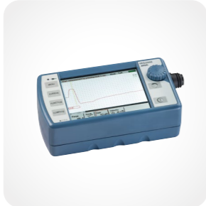
02 / IRG 2000 time domain reflectometer
