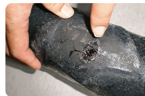
Cable fault on paper-insulated mass-impregnated cable
