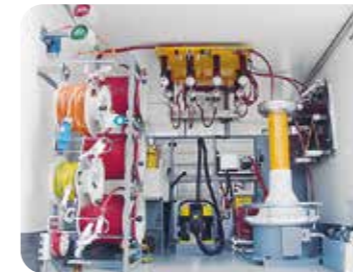
↑ Semi-automatic transcable system, 3-phase, 110 kV
