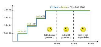
cable insulation. Moreover, partial discharge testing shows and locates the PD faults precisely. The highlight of MWT is the condition-based test duration: Provided it is permitted, the test duration can be shortened, which in turn lowers costs. This way, the cable is only exposed to the increased test voltage for the required duration.
